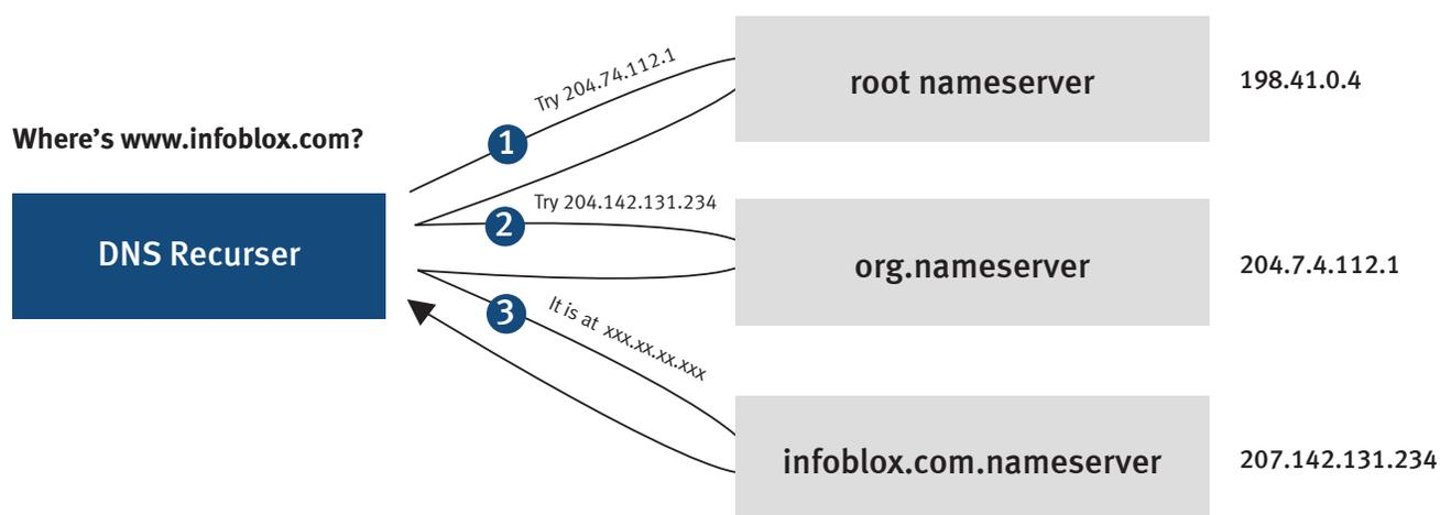
Figure 1: In this example, a recursive name server, labeled “DNS Recursor,” consults three authoritative name servers successively to resolve the address of www.wikipedia.org.
