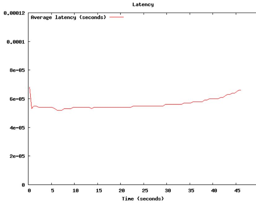
Figure 3: The average query response latency of an Infoblox 4030 remains constant over time.
