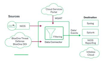
Figure 1: The Infoblox Data Connectorautomatically collects, filters and distributes event information
