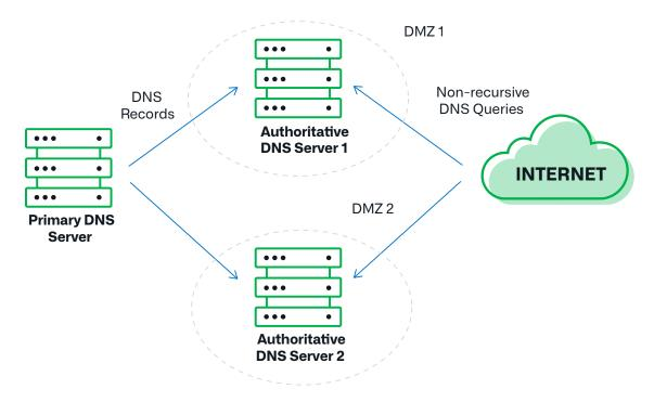
Figure 2: Well-architected external DNS servers
