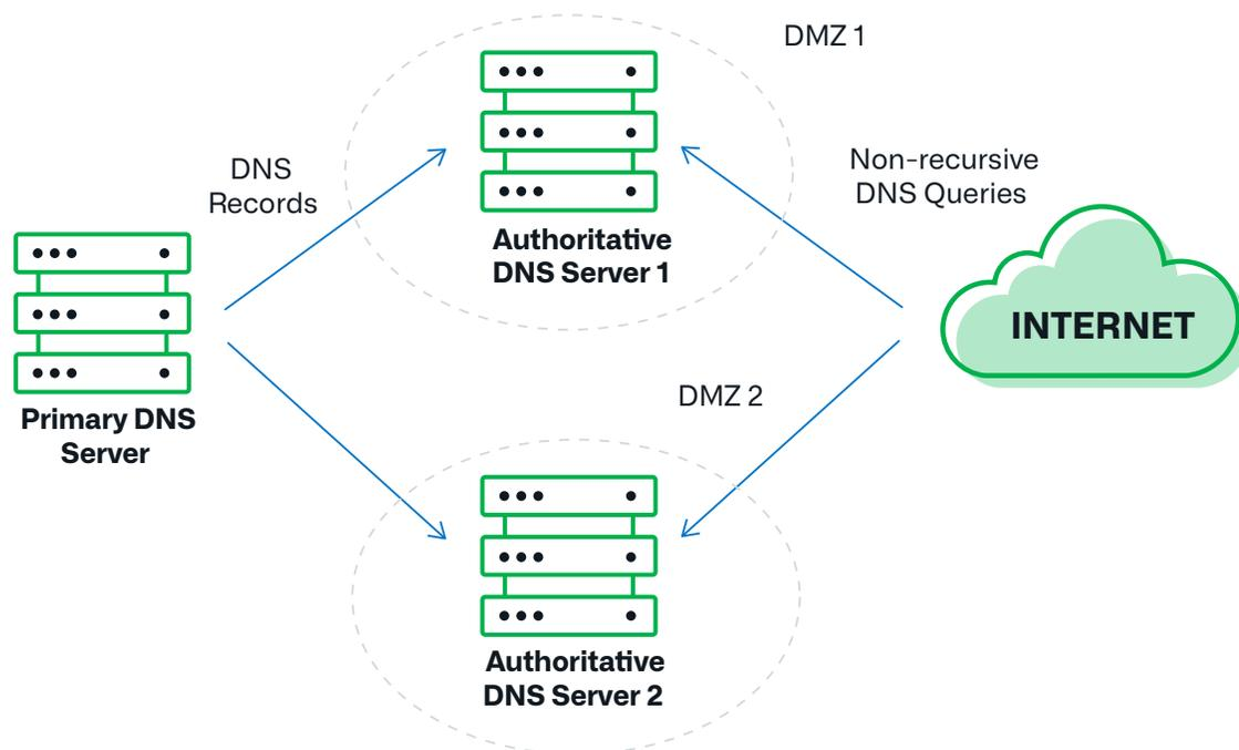
Figure 2: Well-architected external DNS servers
