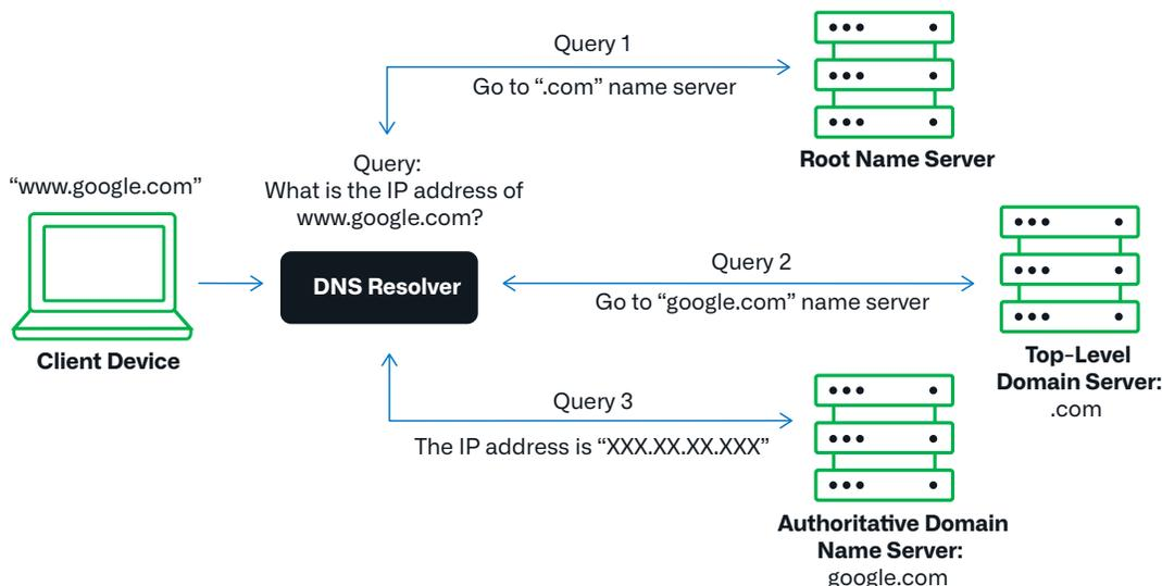
Figure 1: Acquiring an IP address through DNS recursion
