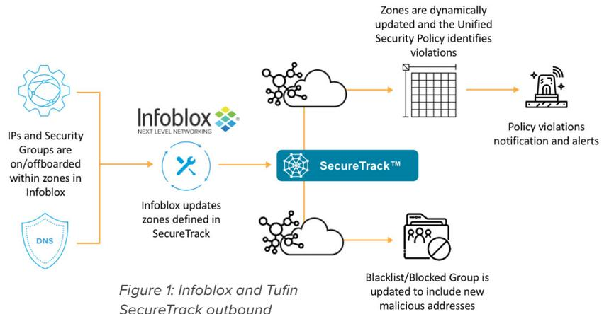
Figure 1: Infoblox and Tufin SecureTrack outbound notification integration.
