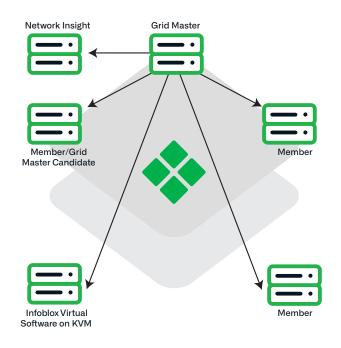
Example of Infoblox Virtual Software for KVM deployed in an Infoblox Grid™
