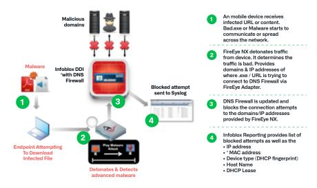
Figure 2: How DNS Firewall works to block malicious connection attempts.
