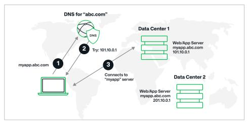
Figure 3: DTC provisioning showing 1) app deployment initiation, 2) company DNS connection, and 3) myapp server provisioning in distributed data centers.
