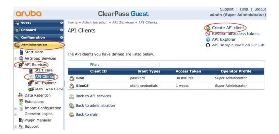
On the "Create API Client" form, add the "Client ID", set the "Operator Profile" to a "Profile" with the correct permissions, set the "Grant Type" to "Client credentials (grant\_type=client\_credentials)" and Remember the "Client Secret" key for later.
