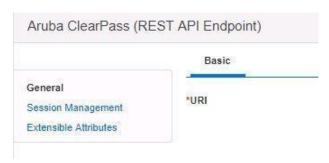
4. In the Session Management settings of the Endpoint, add the "Client\_ID" and "KEY" to the value fields. Note: The Client\_ID is case sensitive and specified on the Aruba ClearPass device as the API Client that was created earlier in this guide. KEY is case sensitive and the Client Secret that was acquired earlier in this guide.
