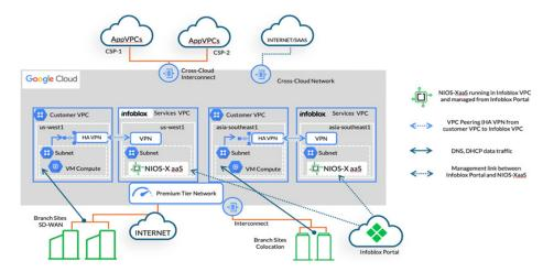
A Cloud VPN Gateway is provisioned within the Google Cloud environment. This gateway acts as the secure ingress point for traffic going to the Infoblox services from the customer's VPC. Within the Infoblox Portal, a new service deployment is configured. The deployment steps include:
